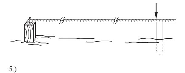
Set a nail into the middle of the center stake. Using a tape or pole, measure the distance from the center stake to points on the perimeter where the forming stakes will be placed.
