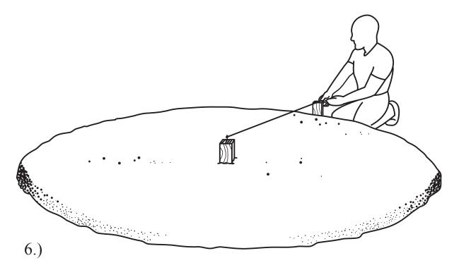
Drive the forming stakes into the ground. All forming stakes should be at the same distance from the center so that a circle is formed. Be sure to allow for the thickness of the forming stakes.
