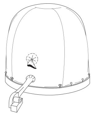
After all workers have exited, roll up and tie off the sleeve, making the Airform as airtight as possible. As placement of Clamp Angles progresses, ventilate under the Airform by starting the inflators. This is especially useful if a large fan is used only for this phase. The EcoShell Inflator must be used to properly inflate the EcoShell's Airform for construction.
