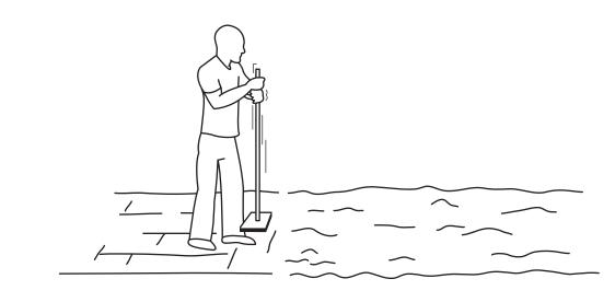
Tamp the ground with a hand tamp or mechanical equipment until it has an even, all-over firmness.
