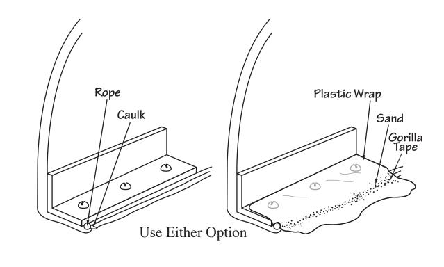
After all Clamp Angles are in place, the joints must be sealed. Clean the joints and seal them with caulking or with plastic wrap and sand. See last page 35 for illustration of Clamp Angle.
