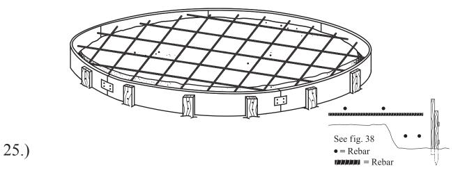
Place floor rebar in the middle of the slab. A cross pattern of #3 (3/8" or 10 mm or 6mm Basalt) rebar 15" (35 cm) on center is adequate for most floors. Stop rebar about 2" (5cm) from edge.
