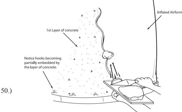
In addition to a Shotcrete pump, the first and subsequent layers of concrete can be hand applied by troweling or flipping it on, using a small mason trowel. Be sure to place only what will stick.
