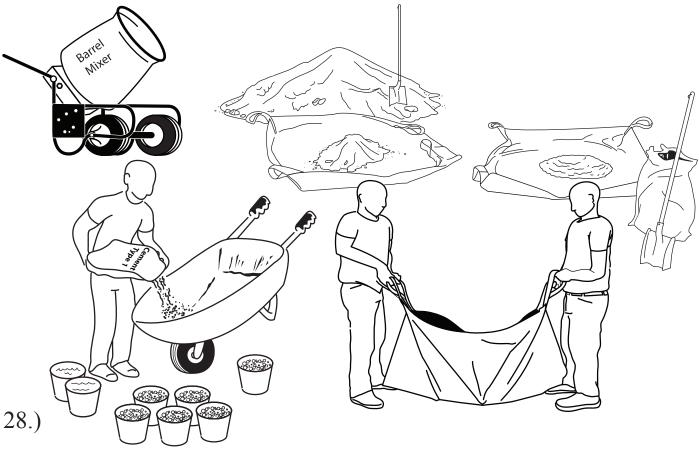
Mix the concrete in a wheelbarrow, barrel mixer, hand mixer or mixing box.
