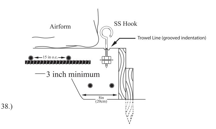
Placement shown is for an EcoShell with a 10' to 20' diameter. Larger structures may require different engineering. Always check for accuracy.
