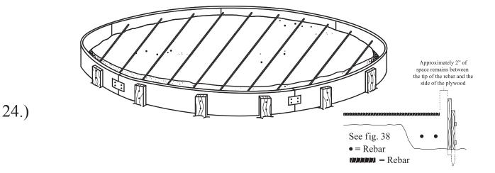
Use bricks to hold perimeter rebar (ring beam tendons) 3" off the dirt and at least 2" in from the formed edge. Then place the floor rebar.
