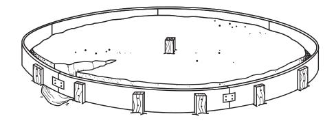
For plumbing, sewer or electrical installations, dig a trench under the plywood perimeter to the spot where the utility will be placed.
