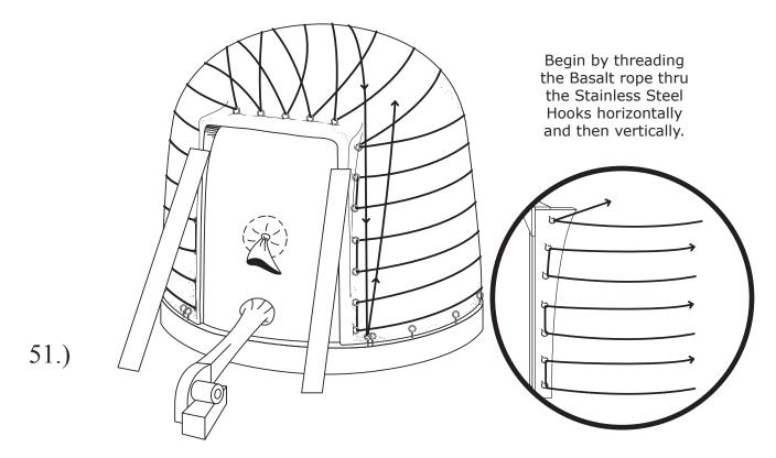
Wrap Basalt rope around EcoShell at 12 inches maximum spacing (30cm). Please use Basalt reinforcing. It will not be destroyed by rusting.
