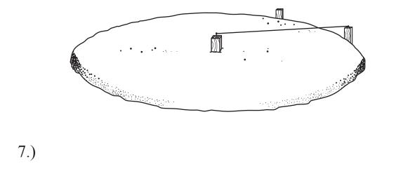
Space the forming stakes about 2 feet apart around the perimeter. That perimeter, created by the forming stakes, outlines the site for the foundation/floor slab edge of the EcoShell.
