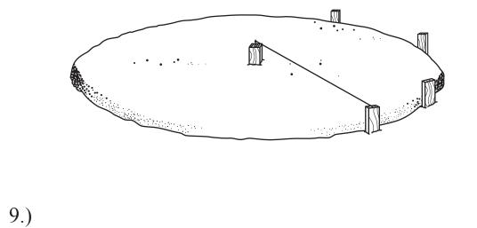
Remember that the forming stakes must all be at the same distance from the center stake plus the thickness of the forming boards. Center stake and forming stakes should all be at the same level.
