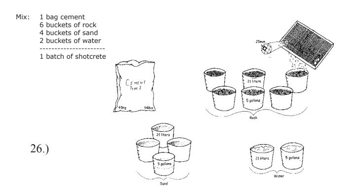
Materials for the footing mix: Cement Type I or II, several 5 gallon (21 liters) buckets, a sifting screen with 25 mm holes.
