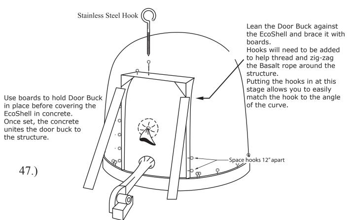
Position door buck to EcoShell and brace it into place with boards. Attach horizontals to verticals. Please use Basalt reinforcing. It will not be destroyed by rusting.
