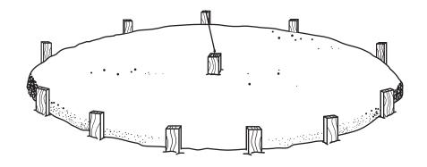
These instructions are for a small to moderate size EcoShell. Larger EcoShells may require deeper and wider footings. After the forming stakes are driven in and leveled, they should get a final diameter check.
