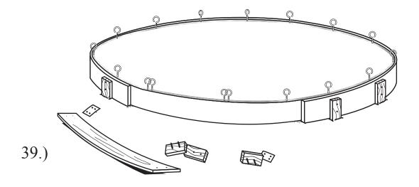
Remove the form boards once the concrete sets -- usually the next day. Provide a safe and clean job site by cleaning and stacking the form boards for future use.
