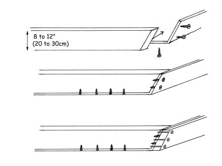
Fasten sheet metal to wood frames with screws or ring shank nails. To minimize leakage, place screws close together. First batch of concrete that's mixed will stop leakage.
