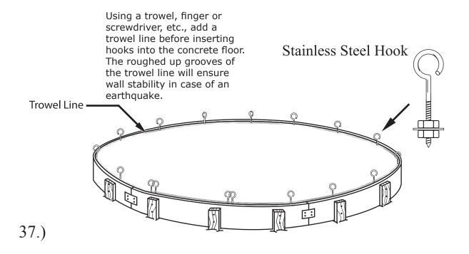
Before the concrete sets, place two hooks on each side of a doorway, but do not place any hooks within the doorway. Dig a small trench approximately 1" (25 mm) wide and 3/4" to 1/2" deep into the fresh concrete between the uprights, except for doorways. For larger structures, this trench should be 2" wide and 1" deep.
