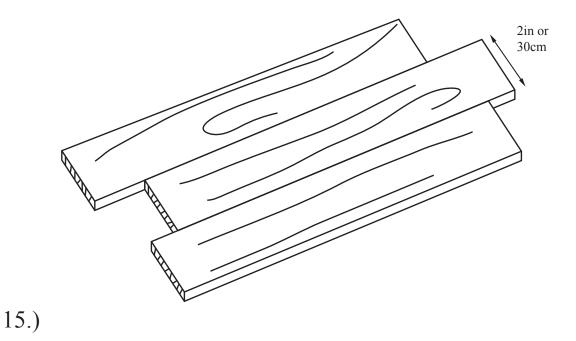
Forming material is needed. Usually this is plywood cut into 12" (30 cm) widths. But many other products, such as heavy sheet metal, plastic panels, siding, etc., will also work.
