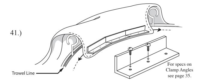
Attach Airform using Clamp Angles as shown. Use 1, 2 or 3 concrete anchors as needed. Anchors can be screws (Tapcons) or a wedge foot anchor. It must be removable.
