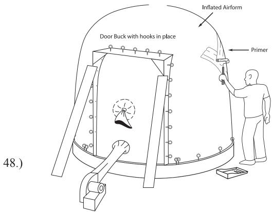
With the augmentation(s) braced against the Airform and the Stainless Steel Hooks in place around the Door Buck, this is a good stage to spray or roll on a light layer of primer over the Airform. The thin, tacky to the touch, layer of primer helps the concrete stick to the Airform.
