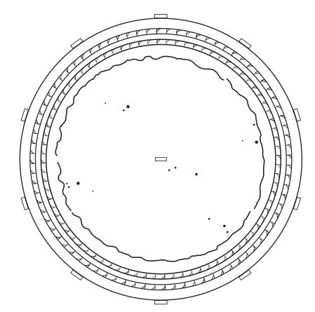
Place two continuous rebars 3/8" (10mm) in diameter into the trench. Rebars may be spliced with a 12" (30 cm) overlap.
