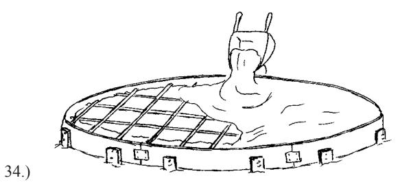
Use care in pouring the concrete so that rebar stays in the middle of the slab. Check to make sure that the placing of the concrete does not knock the forms out of alignment.
