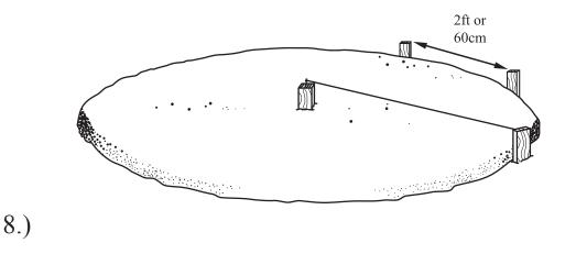
Drive the forming stakes deep enough so that they will hold under the concrete's pressure even after the footing trench is dug around the perimeter.
