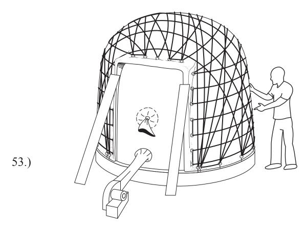
Make a final inspection. Basalt rope should lay flat over the the first layer of cured concrete after being wrapped in a crossing pattern and then a crisscrossed pattern.
