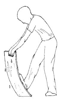
Manually bend the plywood. Before bending, the plywood may need to be soaked for a day or two. Usually, 1/2" (10 to 12 mm) plywood works best.
