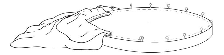
Continue placing Clamp Angles along the guideline. Carefully stretch the fabric along the guideline, distributing the fabric evenly all around. If not stretched evenly, there may not be enough to go all the way around.
