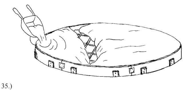
Place concrete. If placing of all of the concrete cannot be done in 15 minutes, start the concrete placing on one side and continue placing by moving across to opposite side.
